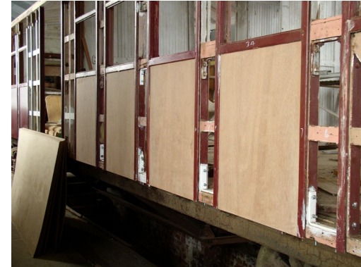
New panelling being fitted to 53RM by DSCR volunteers
